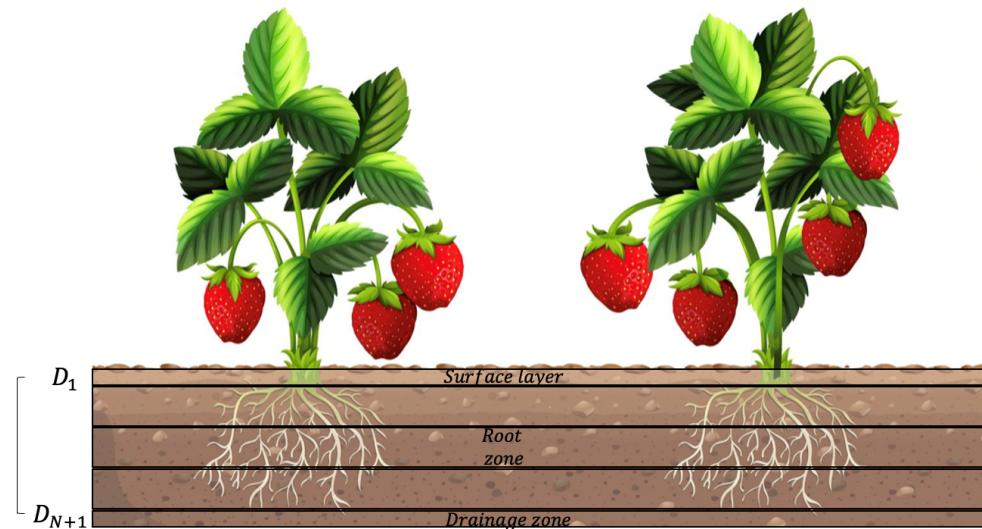
Figure 3. A schematic of the soil layer model with the proposed division into N + 1 layers.
